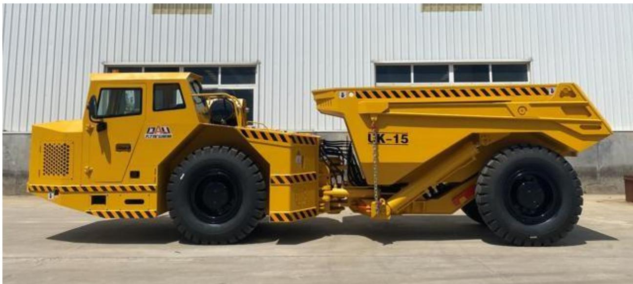
UK-15 is a underground dumper with 15 ton payload for small-to-middle scale mine. Best payload to own weight ratio in its class. It is full of features to help mines maximize tons and minimize costs.
